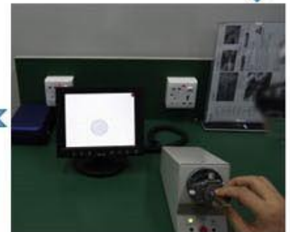
Cleaning end face
