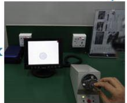
Cleaning end face
