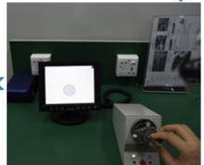
Cleaning end face
