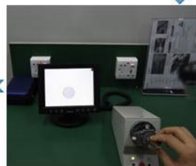
Cleaning end face
