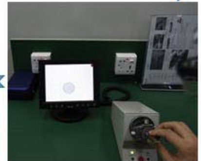
Cleaning end face
