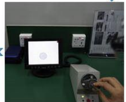
Cleaning end face
