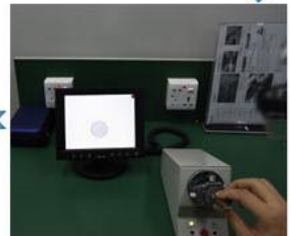
Cleaning end face
